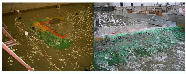
Figure 15: Physical modelling of Western Beaches breakwater armouring (Baird)
