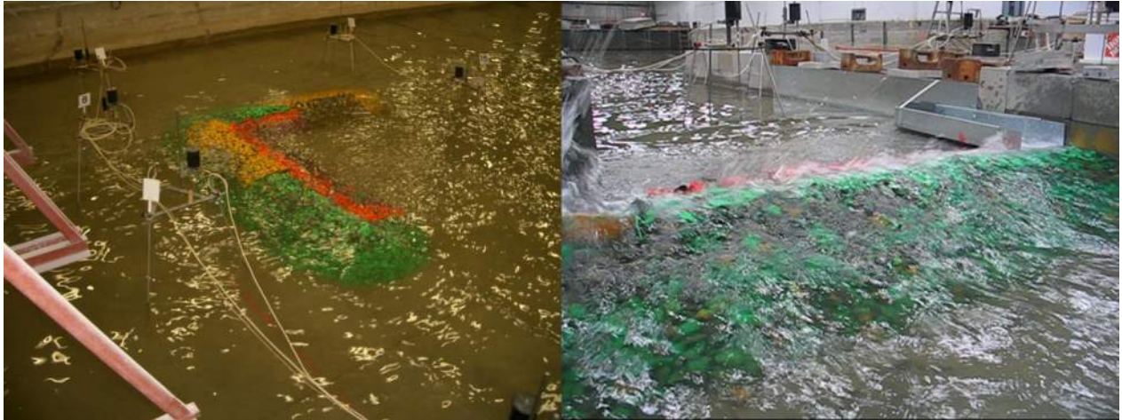
Figure 15: Physical modelling of Western Beaches breakwater armouring (Baird)
