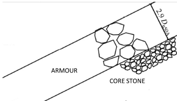
Figure 13: Schematic of multiple layer armour protection
